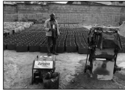
Our new generator & block machine which makes one block at a time.
